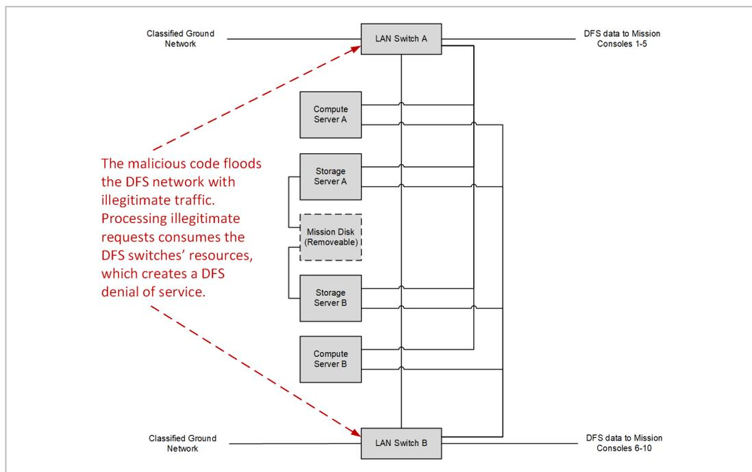
Figure 7: Flooding Attack on DFS Switches
