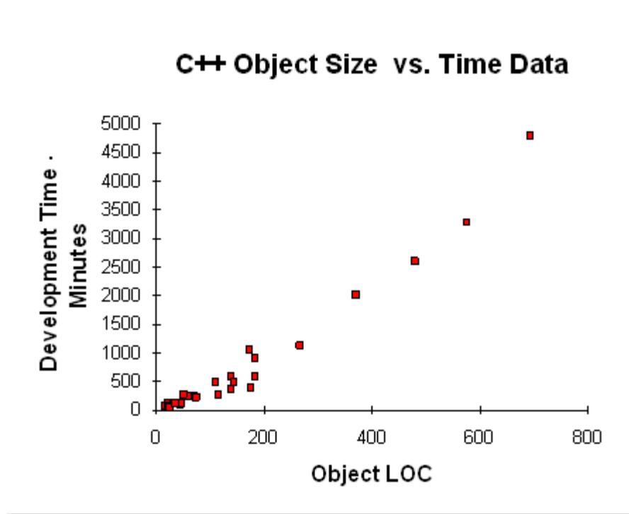
This figure shows the relationship between object LOC and development time for a family of 26 C++ programs. The correlation between size and development time is better than 0.95 and the significance is better than 0.005. Object LOC thus meet the PROBE requirement for close correlation to development effort.
