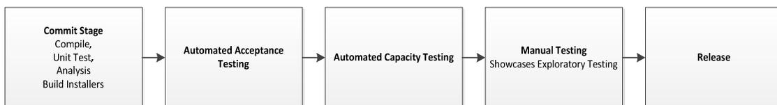
Figure 5: *Continuous Delivery Deployment Pipeline* [Humble 2010]
