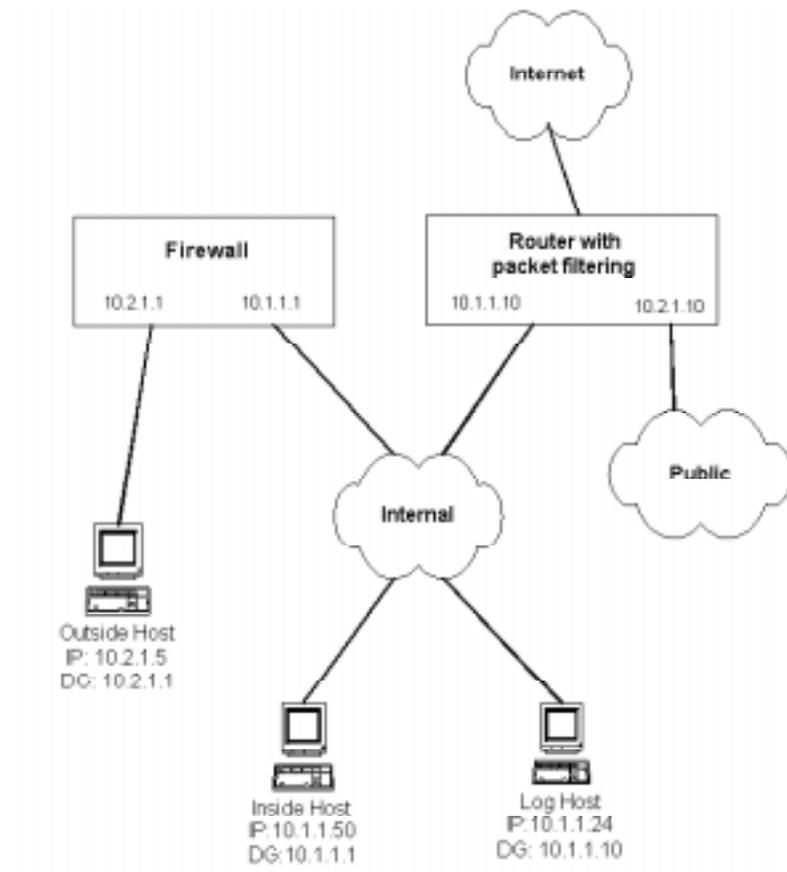
Figure 8-2: Single layer firewall architecture
