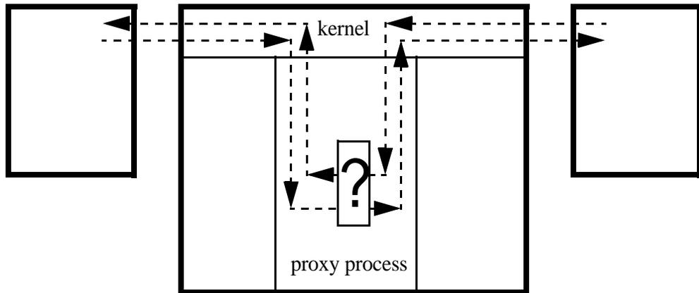
Figure 1-4: Basic border firewall architecture
