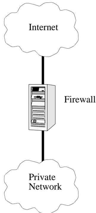
**Figure 1-5: Basic firewall with untrustworthy host architecture**
