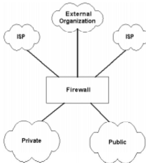
Figure 8-3: Multiple layer firewall architecture
