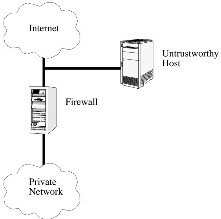
**Figure 1-6: Basic firewall with DMZ network architecture**
