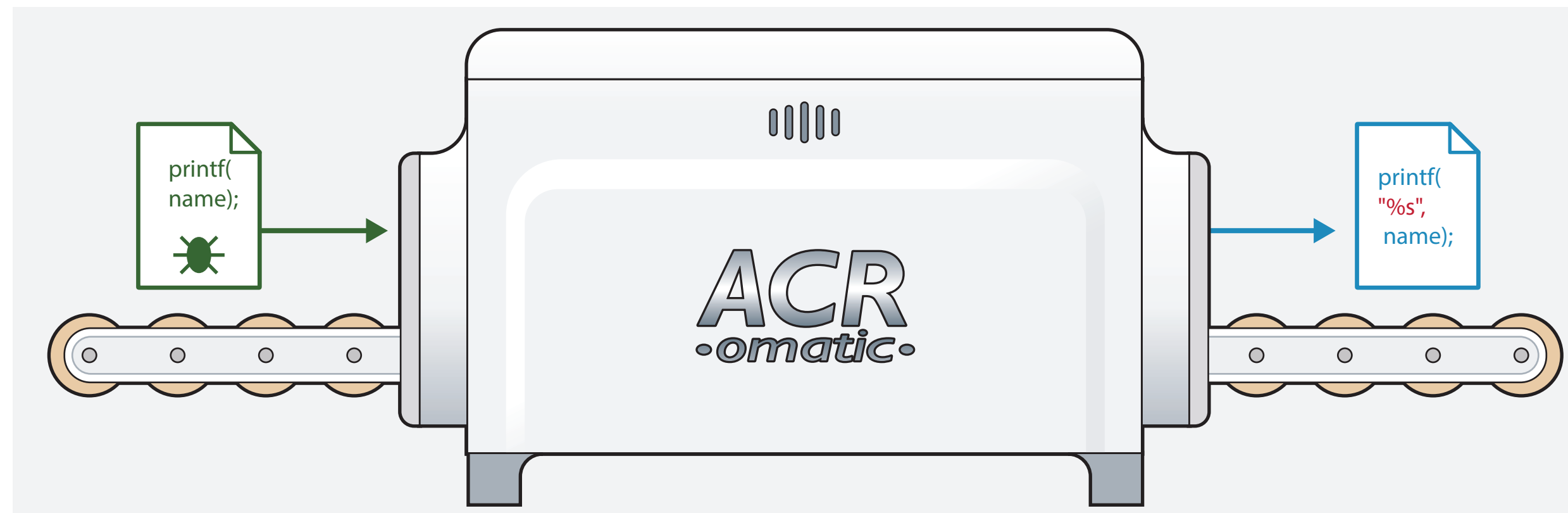
Our ACR tool takes buggy code (shown here, a format-string vulnerability) and repairs the code to remove the vulnerability while preserving the desired functionality of the code.
