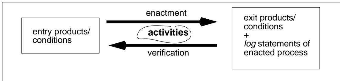
Figure 5-2 Symmetry Between Process Enactment and Verification
