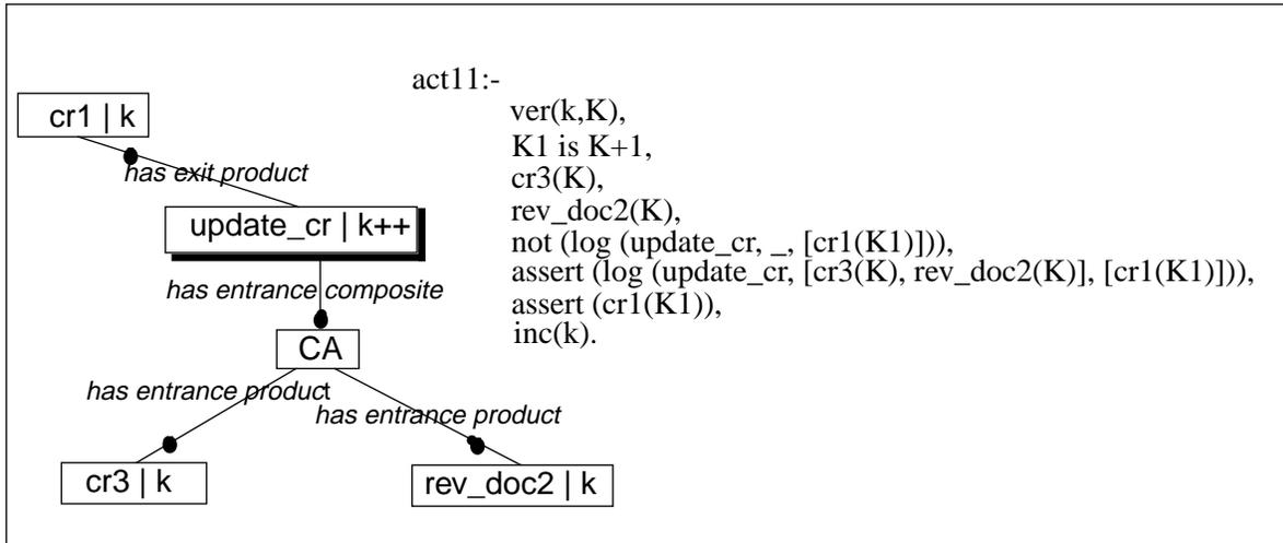
**Figure 4-8 Combining Inputs and Incrementing a Version Number**
