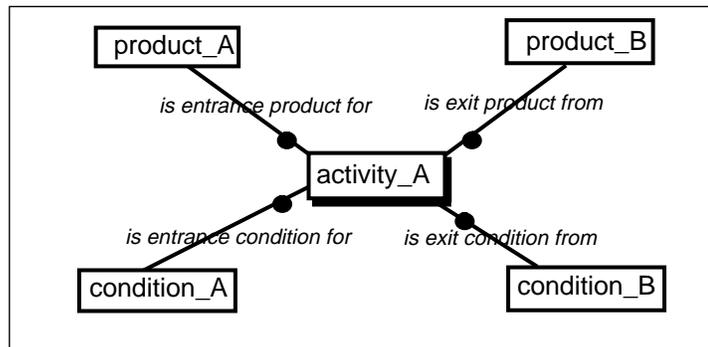
**Figure 3-1 Basic Representation of a Process Element**
